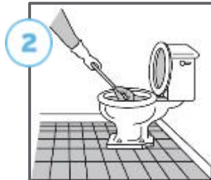
Reduce water level by pushing water repeatedly with brush
