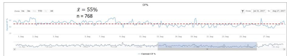
Figure 1: The average cleanliness factor of 55% for August was well below the design cleanliness factor of 85%.
